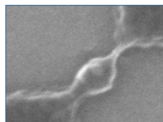
AR-P 679.02 Structural resolution: 6.2 nm gap, 65 nm high
